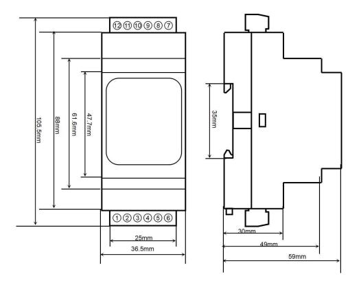
Can be installed on standard DIN35 rails
