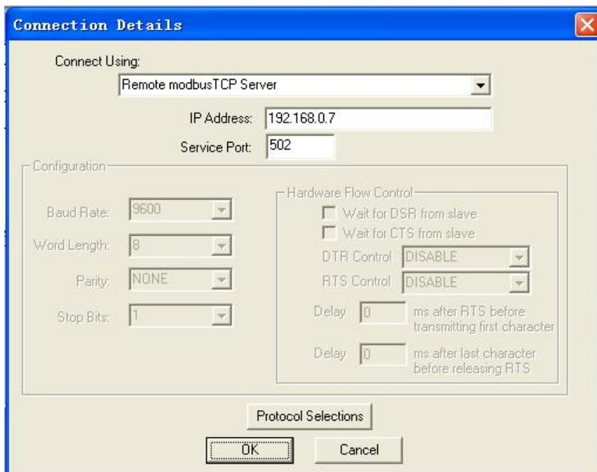
**Figure 5:** Settings for WJ105 using ModScan32 software
