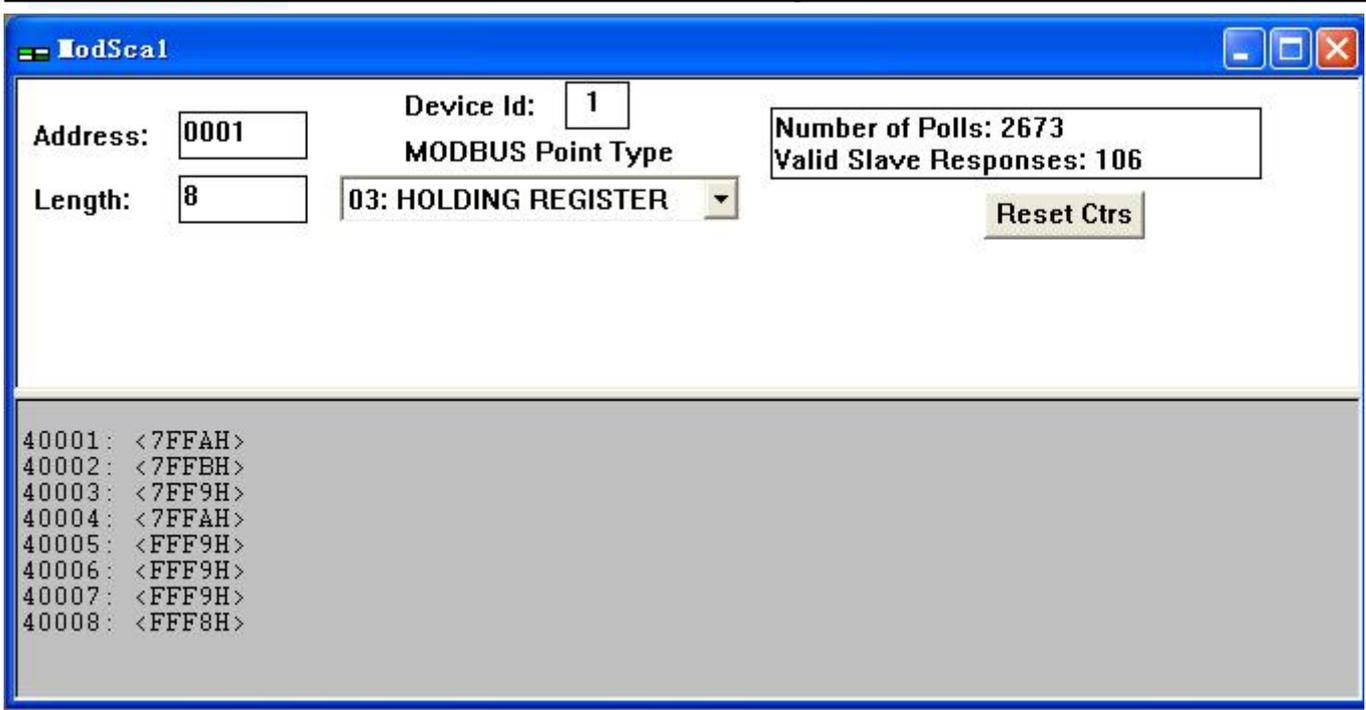
**Figure 6:** WJ105 using ModScan32 software to read existing device data
