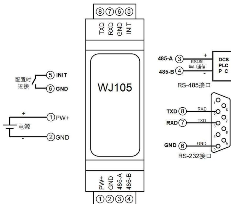
Figure 3 Wiring diagram of WJ105 module
