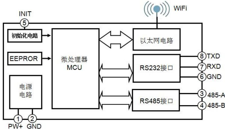
**Figure 2** Internal Block Diagram of WJ105 Module
